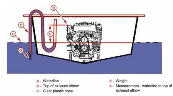
Clear Hose Method for Measuring Exhaust Elbow Height
