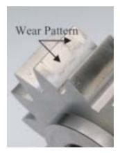
Failure Example: Castrol GPS Passed Stage 12, Failed Stage 13, Total Wear in Stage 13, 300 mm
